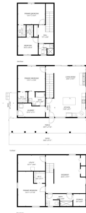
TOTAL: 2136 sq. ft. Basement: 754 sq. ft., 1st floor: 906 sq. ft., 2nd floor: 476 sq. ft. EXCLUDED AREAS: STORAGE: 40 sq. ft., UTILITY: 112 sq. ft., DECK: 57 sq. ft., PORCH: 308 sq. ft., PATIO: 234 sq. ft., WALLS: 169 sq. ft.
